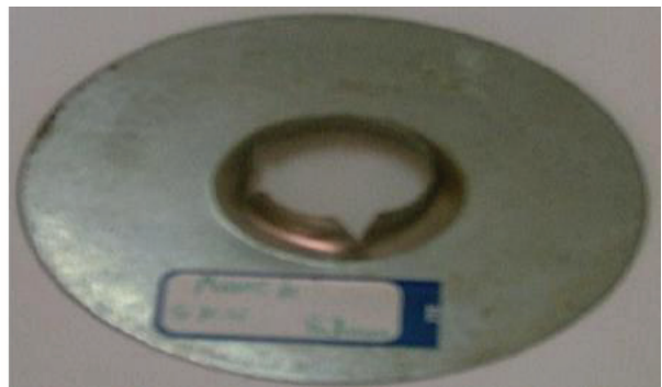
Fig. 23: enlarging with punch 21 mm
