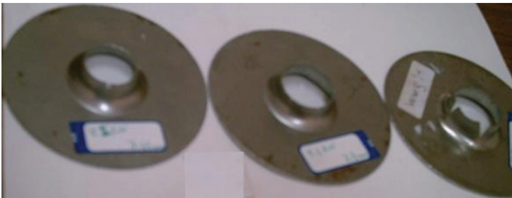
Fig. 17: Typical fractures in the last 3 specimens
