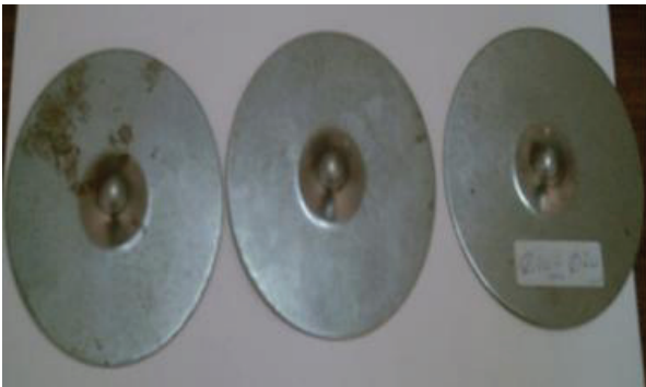
Fig. 7: Photos of beginning and propagation of fractures in forming with a 10 mm diameter punch and 20 mm diameter die
