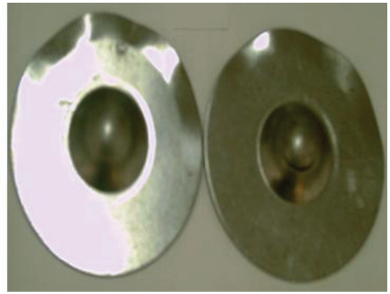
Fig 12: Fractures in Erickson test
