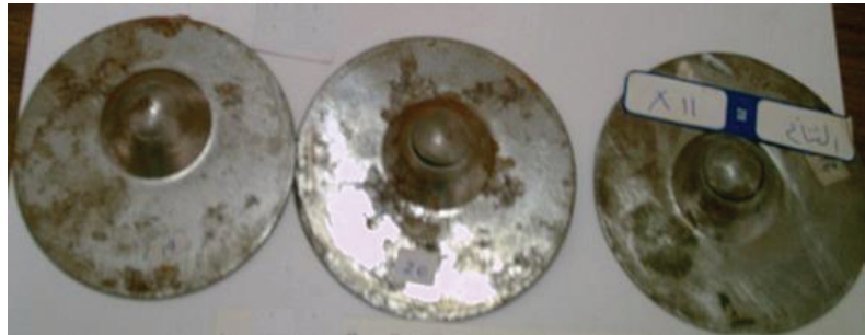
Fig. 13: Fractures on Erickson test
