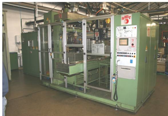
Figure 2. The spin case-hardening device 3KTC.
