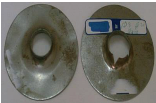
Fig. 22: typical fractures, punch 20 and die 28
