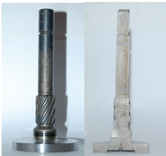
Figure 8. Heat treated shaft (left). Longitudinal cross-section of planetary shaft. Cutting was made with water jet cutting machine. Thickness of hardened case is approximately 1.4 mm (right).
