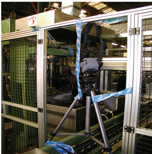
Figure 4. Thermographic camera ThermoCAM PM675.
